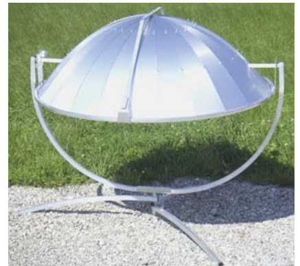
When not in use, the reflector dish will be swing upside down to protect it from rain.
